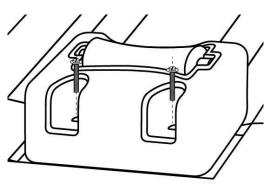
The Bow Stop Roller Assembly Kit is to be placed on bow stop recess area located on the front of the main float. This will raise the noise of your watercraft which adds more weight towards the back. This enables easier launching. If your watercraft keeps on rolling off or will not stay on the float then remove the roller assembly kit. If problem persist then start taking every other set of rollers off on the rails.
